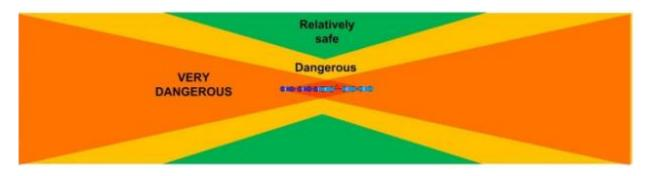
NB: When recovering with a snatch strap or rope, doubling the speed provides 4 times the energy.
